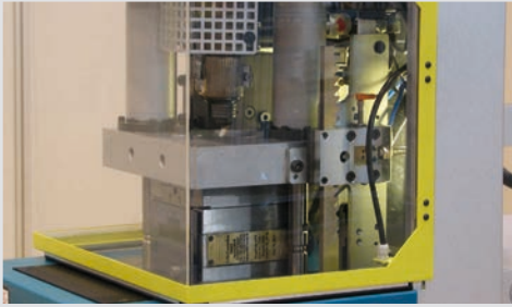
Diagonally arranged tie bars facilitate the installation also of larger moulds
