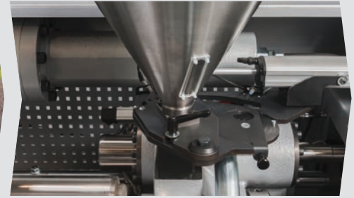
Electrically driven material hopper / feeder for an easier refilling / assembly
